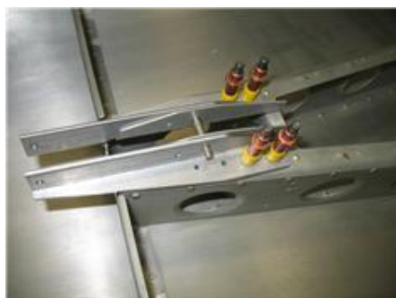
Brackets match drilled to rib, you can see holes in the ribs in photo 3 from previous log entry.
