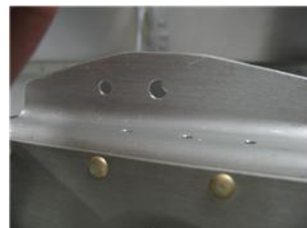
Match drilled AN3 holes on the Dynon bracket to the rib/bracket.
