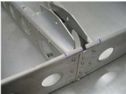
Note bell crank bracket formed into floor ribs. You can see area I had to cut out to fit brackets
