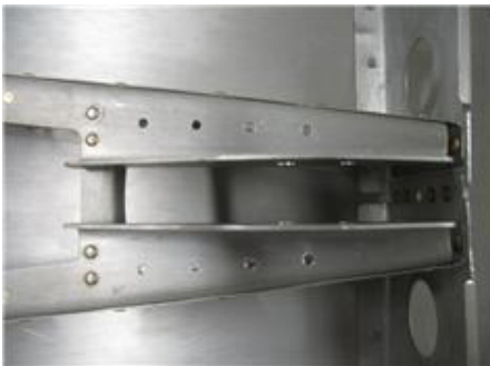
Note support rib rivets on left side of photo, left is forward.
