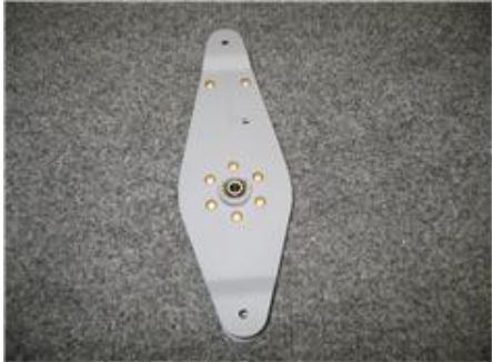
Servo rod connection hole drilled
