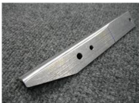
Note: Radius on portion of bracket that nests into existing rib/bracket
