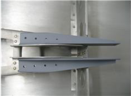
Brackets primed awaiting rivets
