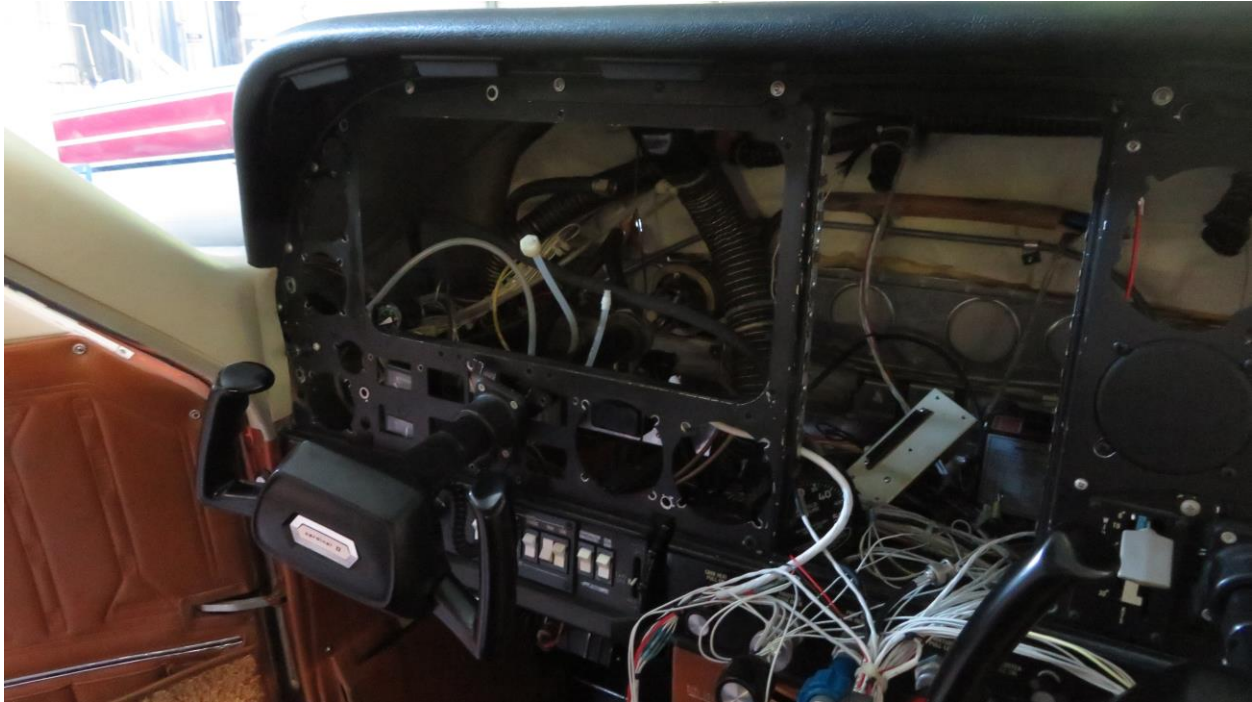
Figure 3 Instrument Chassis and Radio Stack Removed
