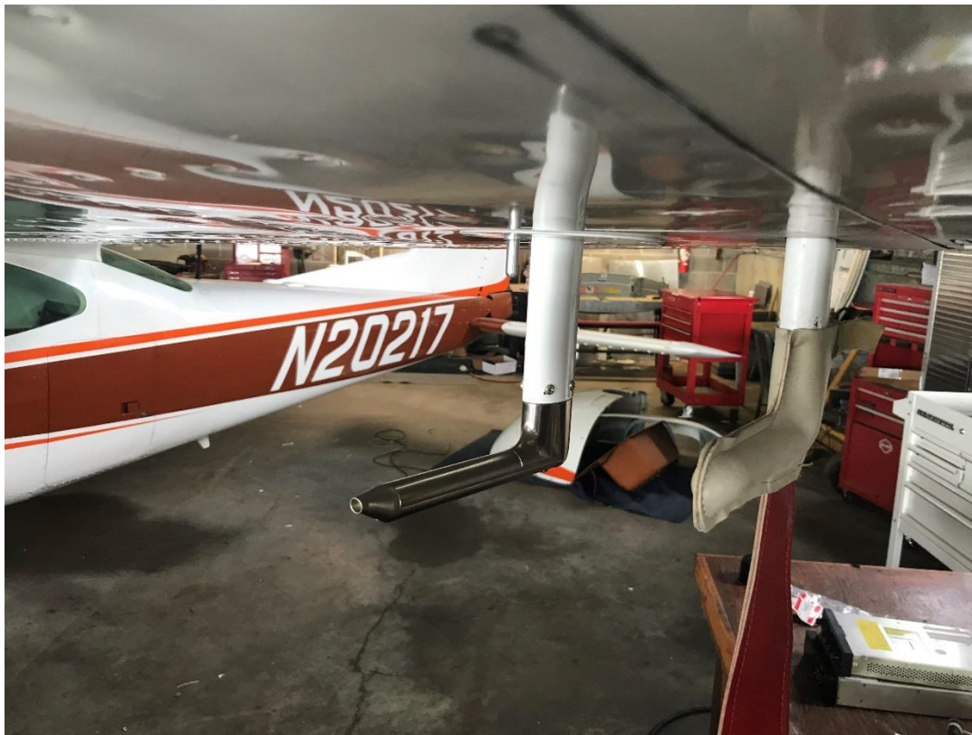
Figure 6 AOA and OAT Probe Installation
