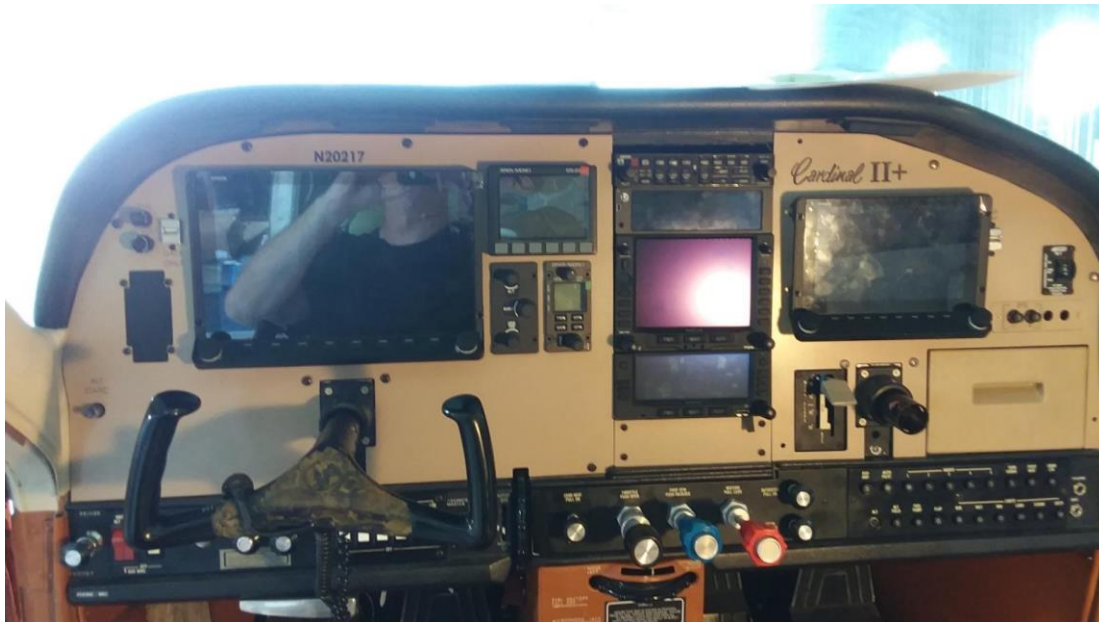
Figure 8 Finished Panel installation
