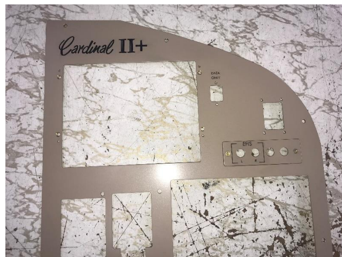
Figure 7 Pilot's and Copilot's Overlay Panels
