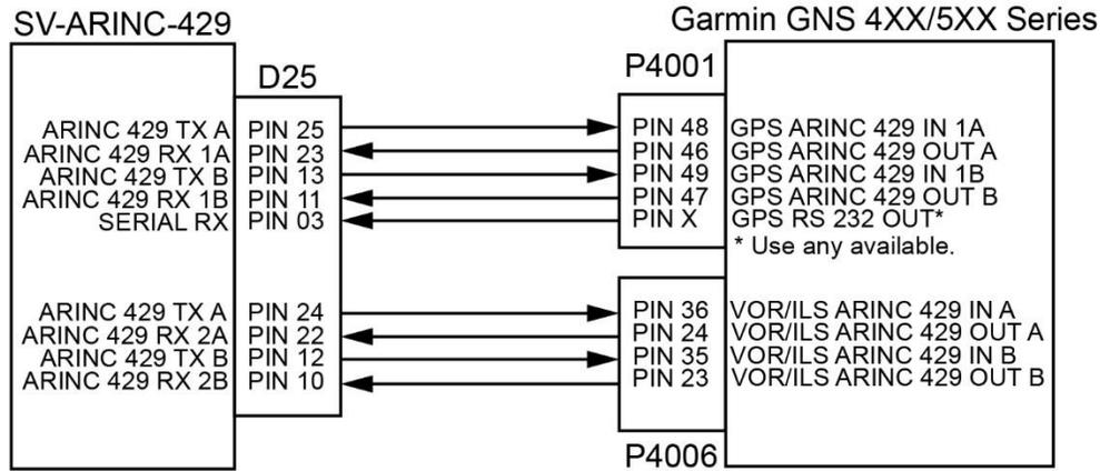
**Figure 2: GNS 4XX/5XX Series to SV-ARINC-429 Electrical Connections**
