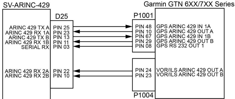
**Figure 3: GTN 6XX/7XX Series to SV-ARINC-429 Electrical Connections**
