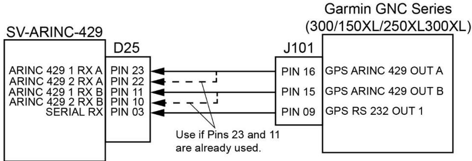
**Figure 5: Garmin GNC Series to SV-ARINC-429 Electrical Connections**
