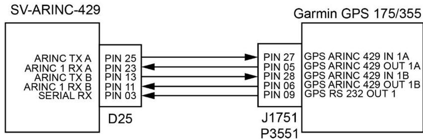
**Figure 6: Garmin GPS 175/355 to SV-ARINC-429 Electrical Connections**
