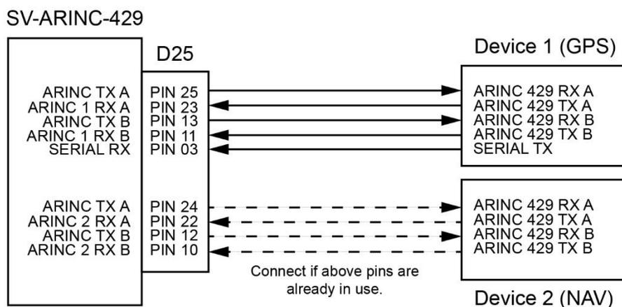
**Figure 1: Typical GPS Navigator to SV-ARINC-429 Connections**
